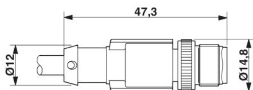
M12 x 1 male connector, straight, shielded
